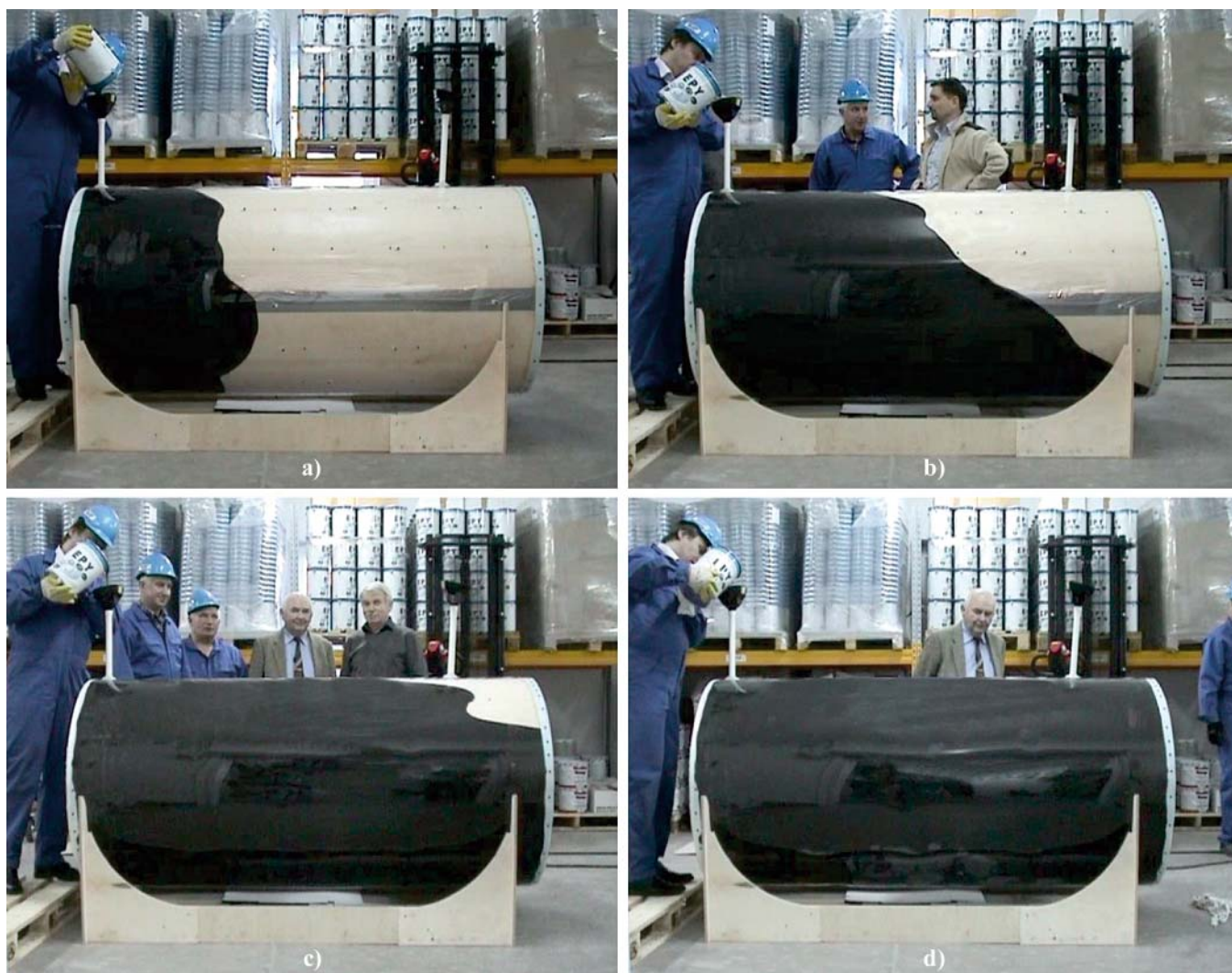
Fig. 4. Model tests of a manner and time of filling the pouring gap between shaft and sleeve with liquid EPY resin compound
