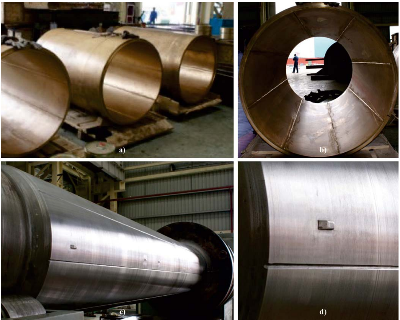
Fig. 5. Sections of the bearing sleeve and the shaft with cut splineways and welded spacing elements
