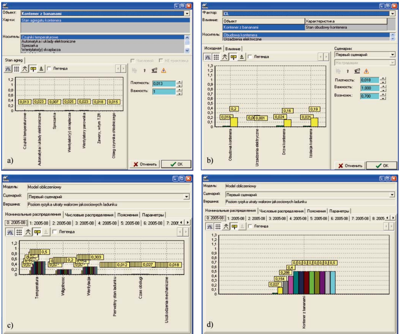
Fig. 4. Dialogue windows showing particular calculation phases: a) dialogue window for inserting fuzzy measures into gradations of characteristics of examined objects; b) dialogue window for inserting power of impact of risk factor onto object of examination; c) dialogue window showing temporary results of calculations in peaks of 2nd layer of the conceptual model; d) dialogue window showing results of calculation of integral risk level of loss of refrigerated cargo quality merits. Source: the author's original elaboration
