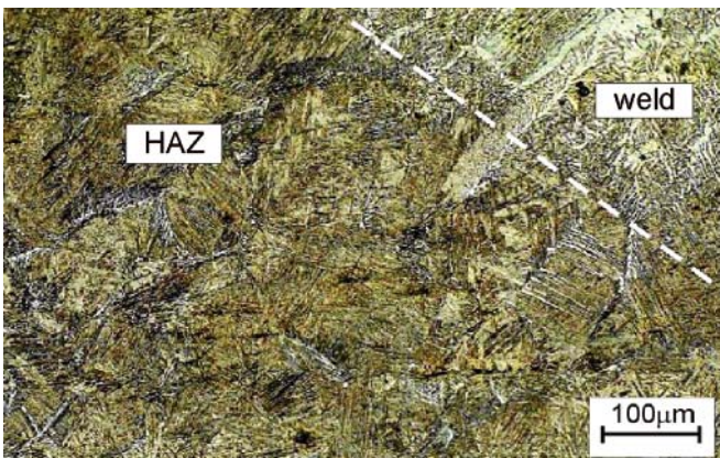
Fig. 9. The microstructure of MI sample (M21 shielding gas, heat input of 0.90 kJ/mm): coarse-grained structure in the HAZ, quasi-pearlite and acicular bainitic structure, visible small bands of ferrite
