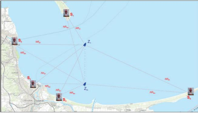
Fig. 3. Bearing measurement structure (source: own work)
