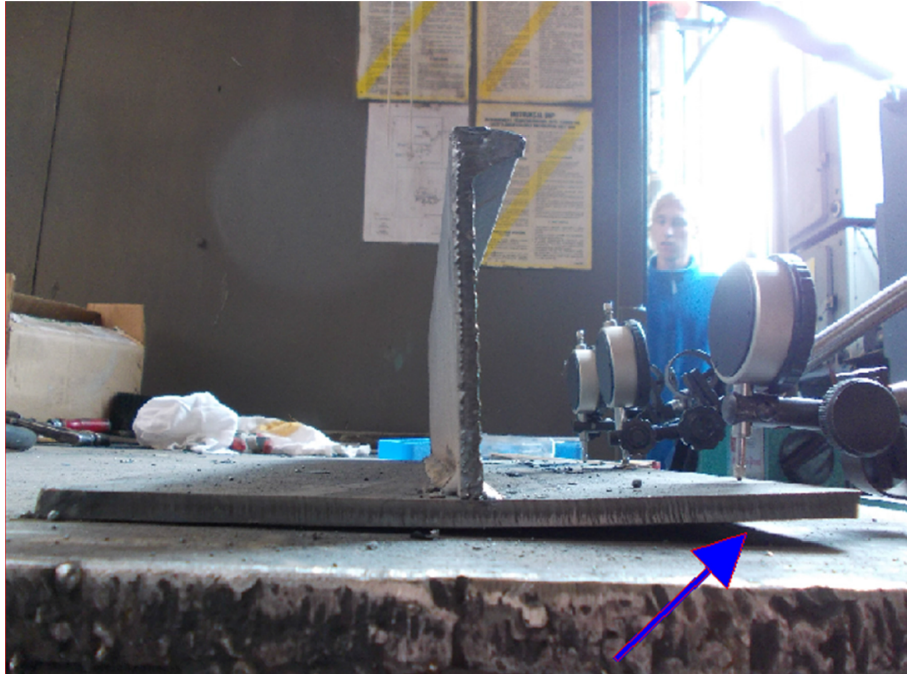
Fig.4. Measurement of angular deformation
