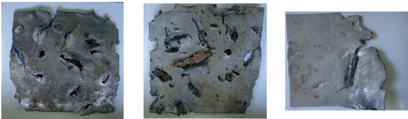
Fig.9. Effects of 7020M alloy sheet perforation (dimensions 300x3000): a) homogeneous g = 12 mm b) split (w-inner, z -outer from the source of explosion, total thickness g = 2x6 mm) after detonation of high explosive shell of OF412 type and calibre 100 mm with the contents of 1,4 kg of TNT, taking place at a distance of 0,6 m.
