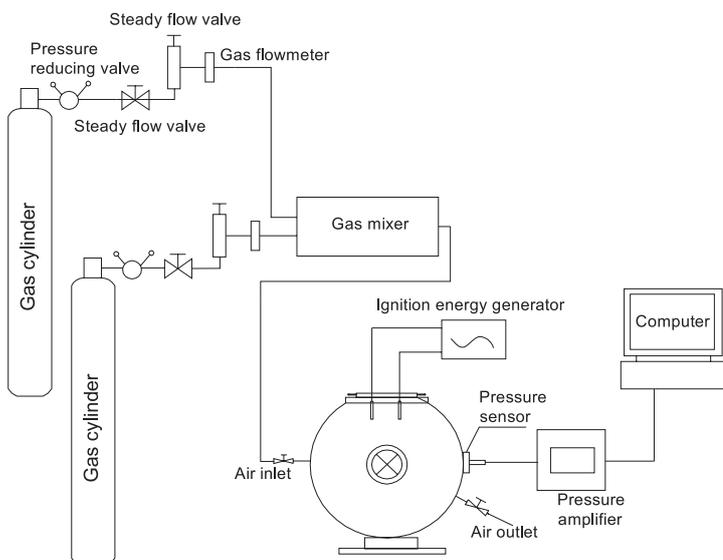
Fig. 7 The device of explosion experiment
