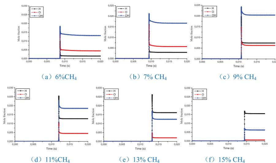
Fig. 6 Trend of free radical change in gas explosion process
