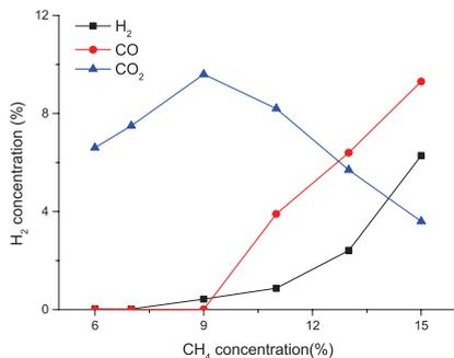
Fig. 8 Trend of gas product after gas explosion
