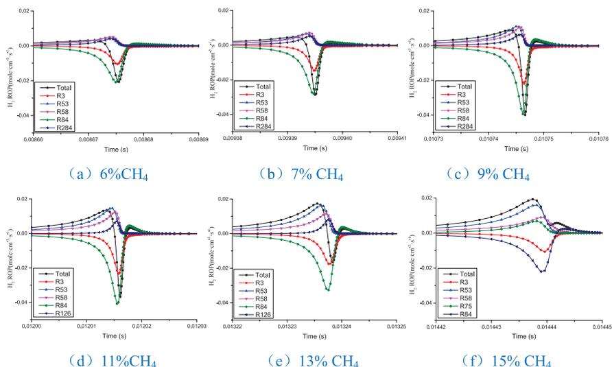
Fig. 5 Key basic element reaction step of gas explosion  $H_2$
