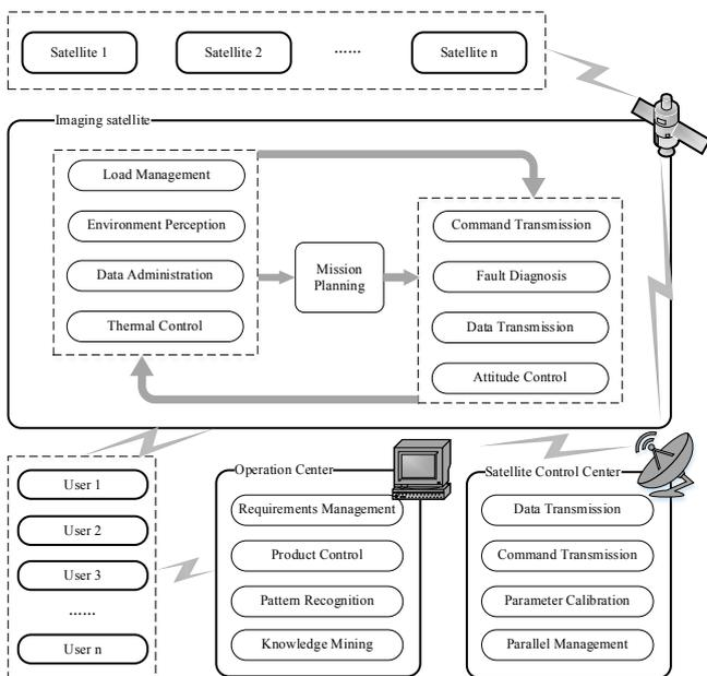
Fig. 3 Framework of the proposed Earth observation system
