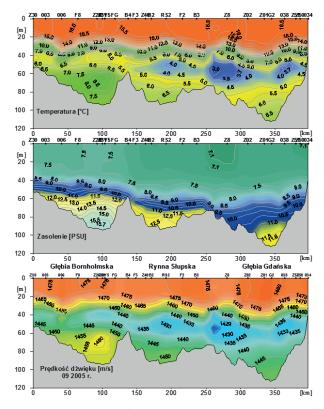
Fig. 4. Vertical distribution of temperature, salinity and sound velocity profile on the hydrological profile though the depths of the southern Baltic sea (September 2005)
