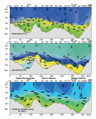
Fig. 2. Vertical distribution of temperature, salinity and sound velocity profile on the hydrological profile though the depths of the southern Baltic sea (February 2005)
