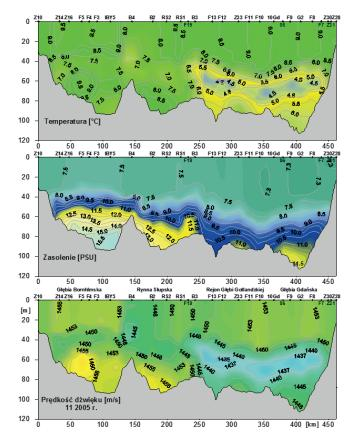
Fig. 5. Vertical distribution of temperature, salinity and sound velocity profile on the hydrological profile though the depths of the southern Baltic sea (November 2005)
