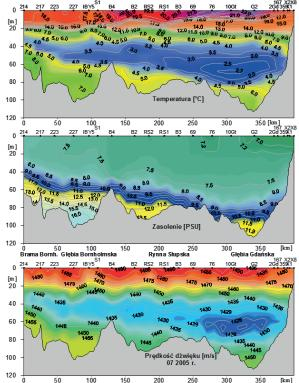
Fig. 3. Vertical distribution of temperature, salinity and sound velocity profile on the hydrological profile though the depths of the southern Baltic sea (July 2005)
