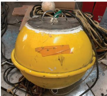
Fig.2 Photo of the wave height meter
