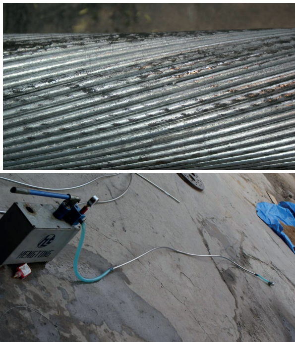
Fig. 13 Broken-out section view of umbilical after test
