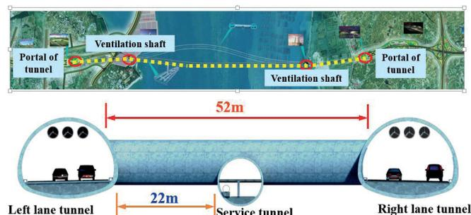
Fig. 2. Schematic diagram of the cross-section of tunnel layout
