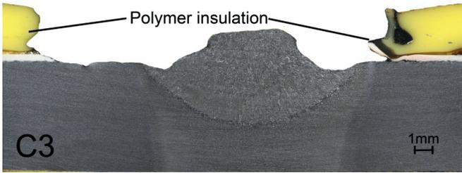
Fig. 2. Macro cross-section of the welded specimens C1, C2, C3 (insulated specimen C). Etch. Nital
