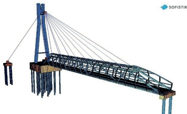
Fig. 4. Visualisation of the FEM model used in the analysis
