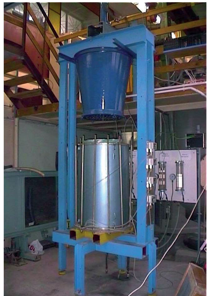
Fig. 3 Calibration chamber at GUT [24]
