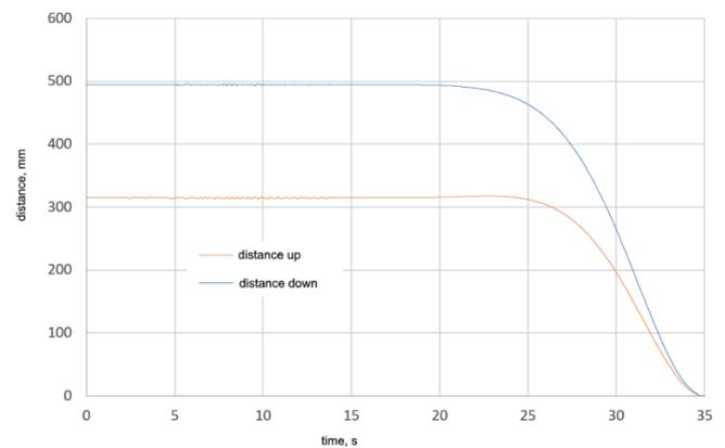
Fig. 14. Distance between fire damper and frame in upper and lower part
