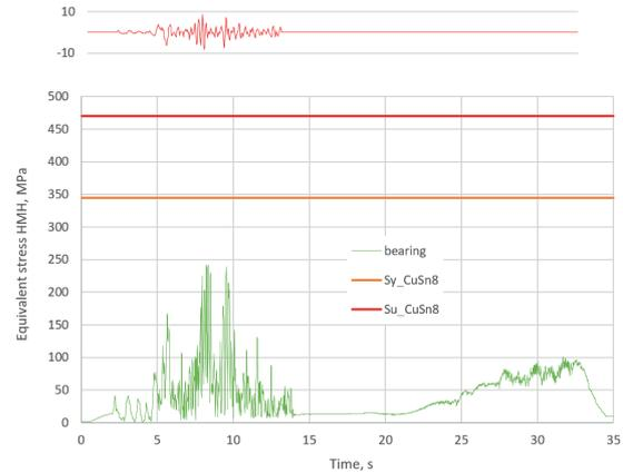
Fig. 9. Equivalent stress history in parts made of CuSn8 bronze
