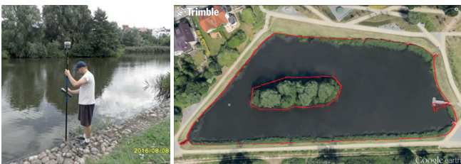
Fig. 11. Staking out the coastline point (left) and the coastline of the retention reservoir, measured and obtained from the Google Earth Pro platform (right) (own study).
