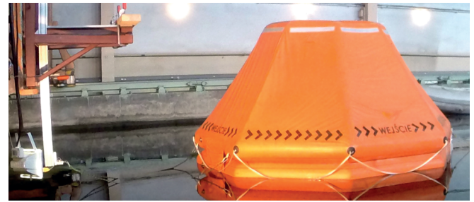
Fig. 4. Model test of the novel life raft tied to the carriage, loading condition: 1 person, V = 0 \text{ m/s}
