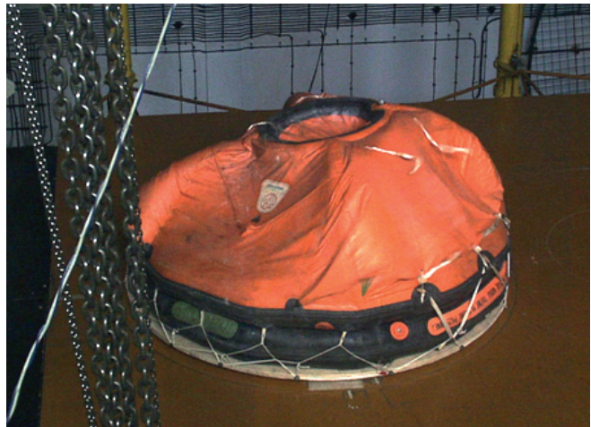
Fig. 1. Deformation of the canopy of a 6- person life raft - real scale tests in the wind tunnel of Institute of Aviation , Warsaw, Poland [4]
