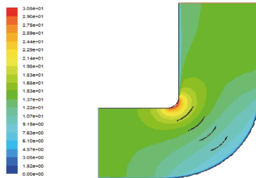
(c) Four baffles arranged disaggregated
