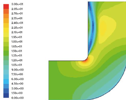
Fig. 6. The velocity distribution of the flue gas in the non-deflector plate
