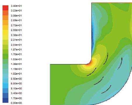
Fig. 14. The velocity field profile of the different deflector plates
