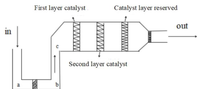
Fig. 1. Simplified diagram SCR catalytic reaction system
