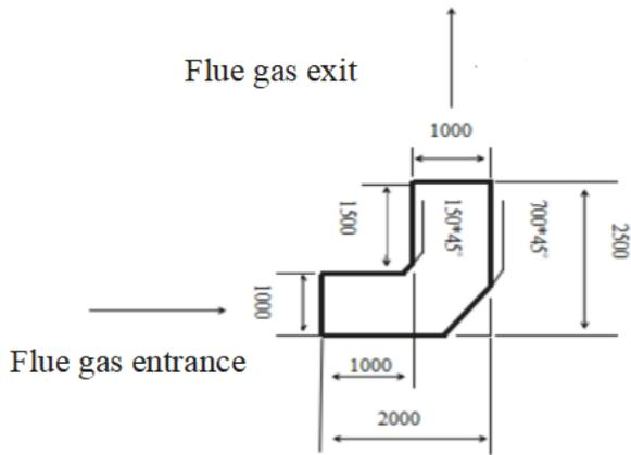
Fig. 2. Inclined type flue structure diagram (no guide plate)
