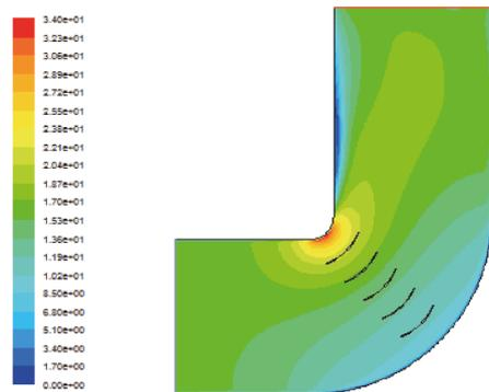
(e) Five points out baffle arrangement (after the first two three)
