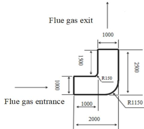
Fig. 5. Circular flue structure diagram (no guide plate)
