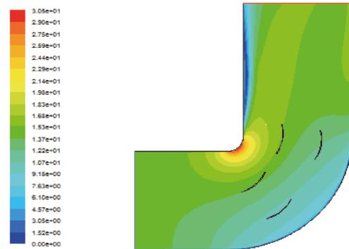
Fig. 8. The velocity field profile of the different deflector plates
