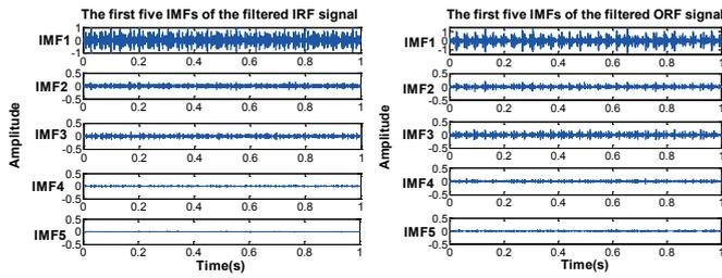
Fig. 9. The first five IMFs of the filtered IRF, ORF and REF signals; (a) The first five IMFs of filtered IRF signal; (b) The first five IMFs of filtered ORF signal; (c) The first five IMFs of filtered REF signal
