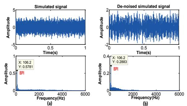
Fig. 2. The simulated inner fault signal; (a) The time domain and envelope spectrum of the simulated inner fault signal; (b) The time domain and envelope spectrum of the de-noised simulated signal which is obtained by the proposed method
