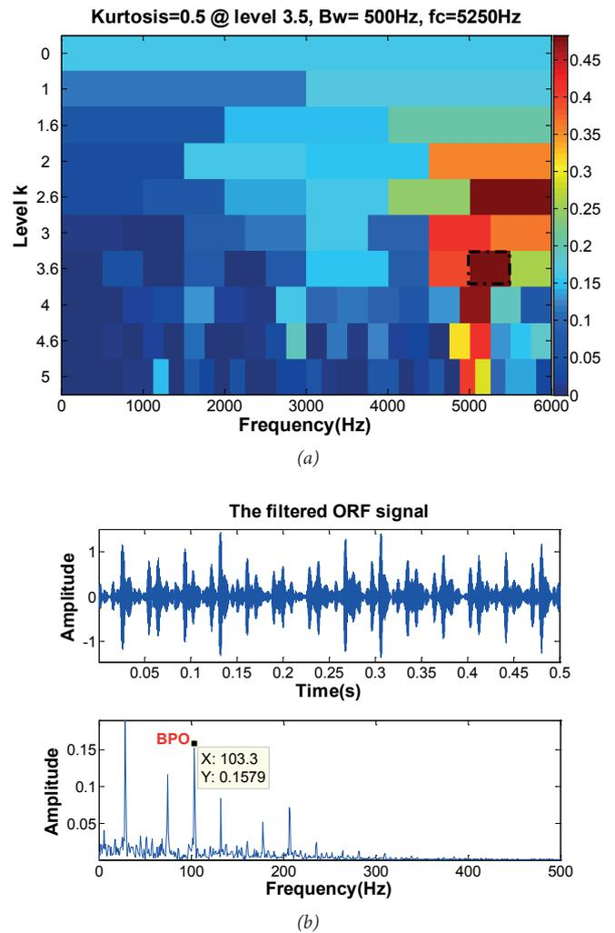
Fig. 7. The results of ORF signal by SK. (a) The 2-D SK of ORF; (b) The filtered ORF and its envelope spectrum
