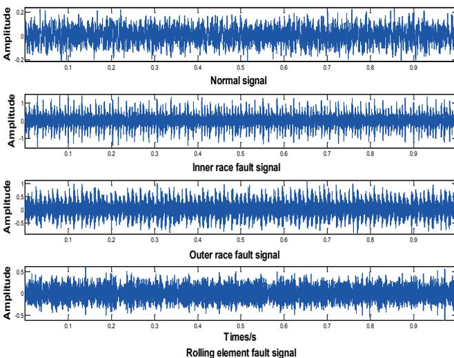
Fig. 4. NORM signal and IRF, ORF, REF fault signals
