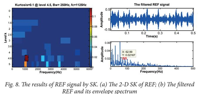
Fig. 8. The results of REF signal by SK. (a) The 2-D SK of REF; (b) The filtered REF and its envelope spectrum
