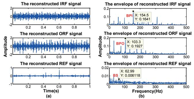
Fig. 10. The reconstructed signals and their envelope spectrums
