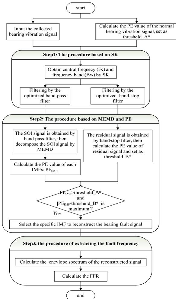
Fig. 1. The processing procedure of the proposed method
