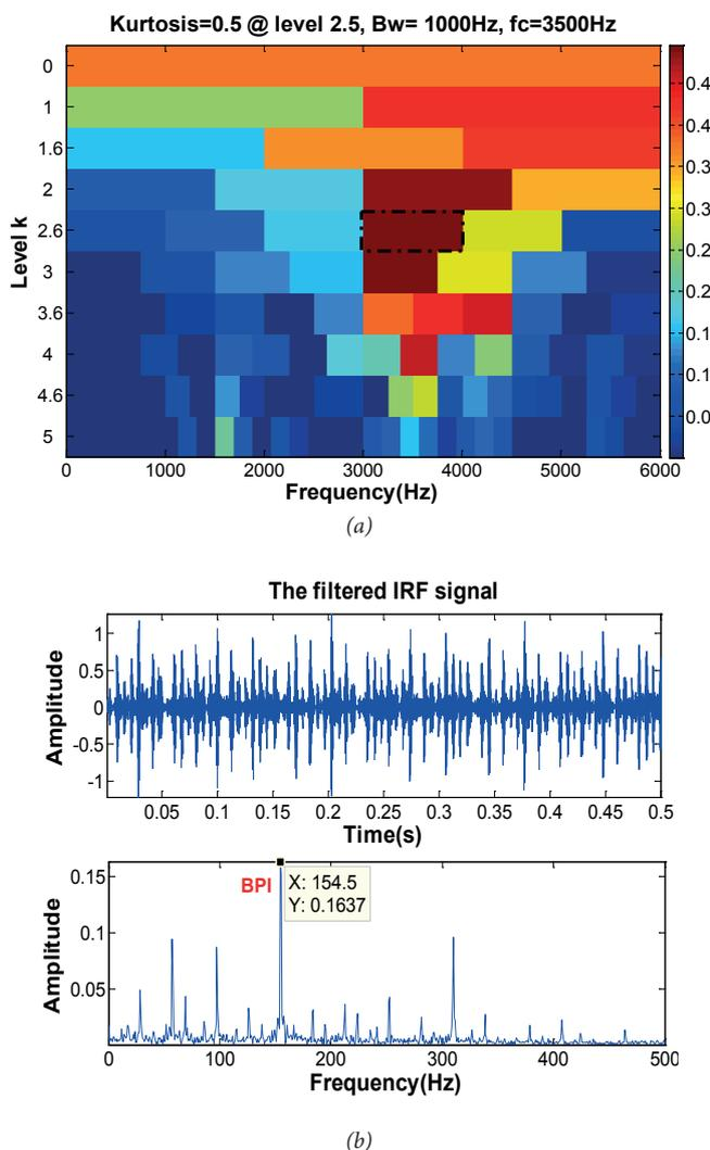
Fig. 6. The results of IRF signal by SK. (a) The 2-D SK of IRF; (b) The filtered IRF and its envelope spectrum
