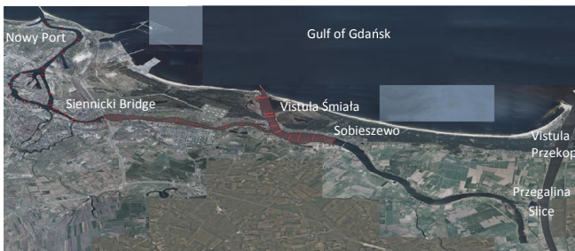
Fig.1. Dead Vistula with available cross-sections (red lines) and the adopted computational area (area shaded in red) (source: ortofotomap from http://mapy.geoportal.gov.pl )
