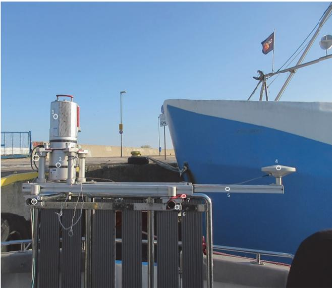
Fig. 3 Components of the Riegl VMZ-400 system on a vessel
