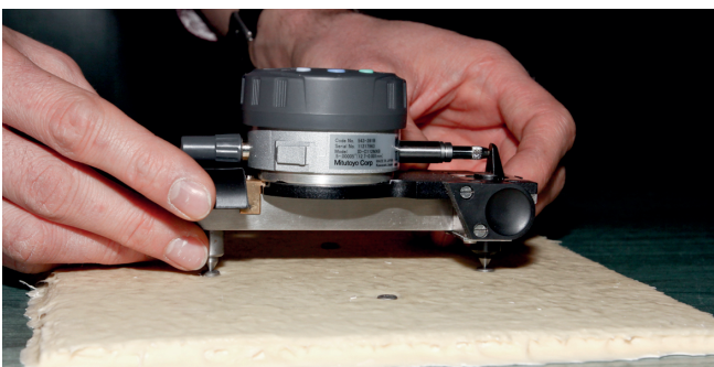
Fig. 5. Extensometer used for length change measurement
