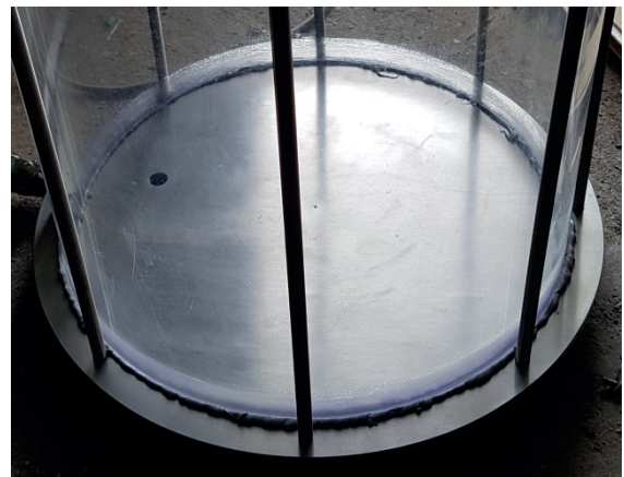
Fig. 8. Sealing of lower tank
