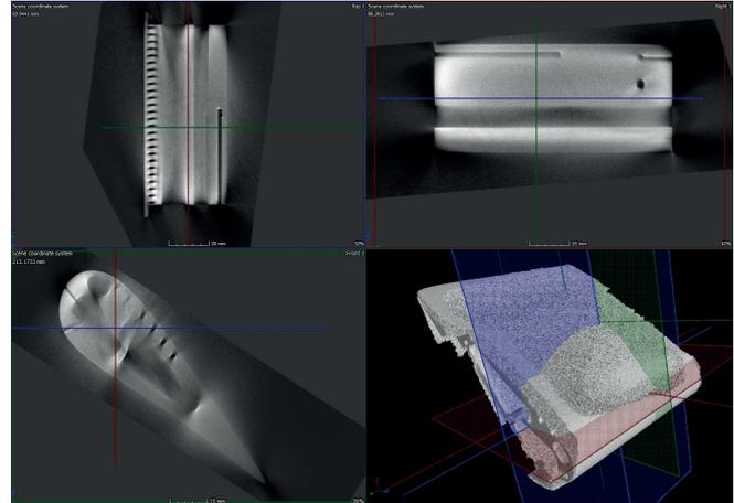
Fig. 3. Exemplary images of cross-section of turbine blade model
