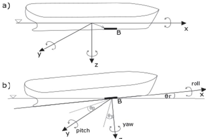
Fig. 10. Ship motions caused by sea surface waving
