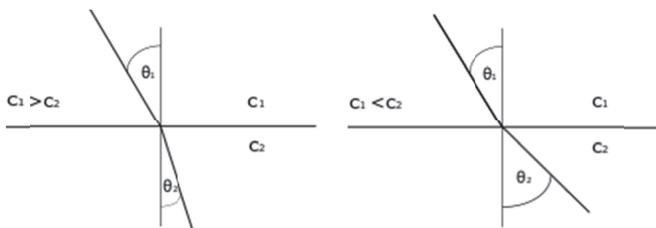
Fig. 6 Refraction principle
