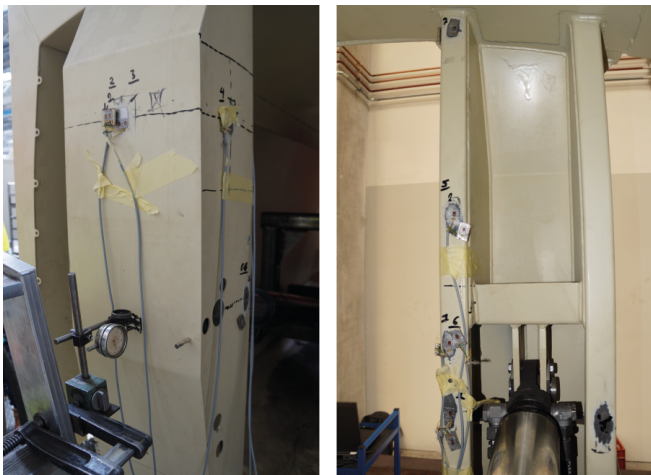
Fig. 7. Location of the strain gauges on the real structure
