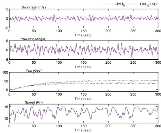
Fig. 3. Responses of the uncontrolled autopilot system
