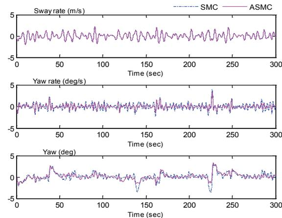
Fig. 4. Simulation results of sway and yaw
