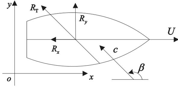
Fig. 1. Definition of added resistance and drift force
