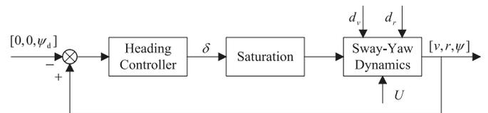
Fig. 2. The autopilot control system
