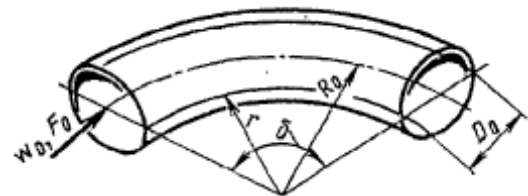
Fig. 2.2. Curved section of pipe [10]
