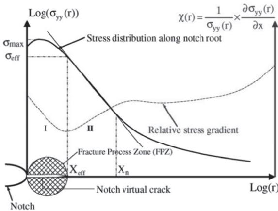
Fig. 1. Stress distribution and relative stress gradient [1]
