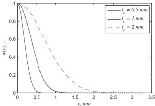
Fig 3. Weight function and different values of critical length [8]
