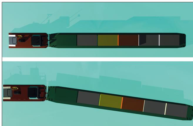
Fig. 7. Turning performance of convoy: BM-500 and BP-500, turning control by bow steering system and dynamic coupling
