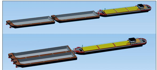
Fig. 4. Convoy of BM-500 and 2 BP-500 barges: up-river configurations (upper drawing) and down-river configurations (bottom drawing)
