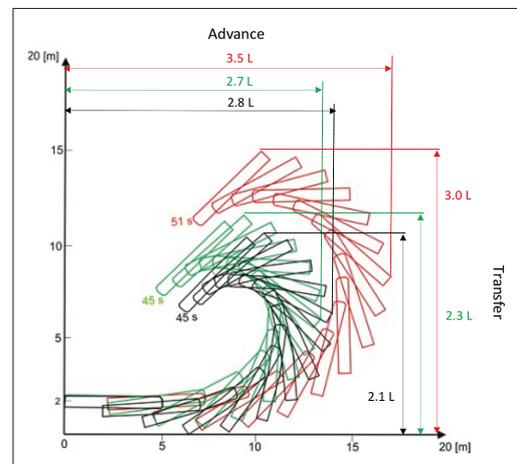
Fig. 6. Turning manoeuvre of the push train using bow rotors (red), stern rudders and bow rotors (green), stern rudders, bow rotors and dynamical coupling system (black)
