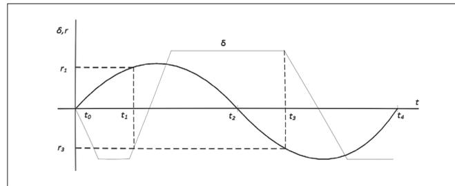
Fig. 5. Diagram of the evasive manoeuvre,  $\sigma$  – rudder angle [°],  $t_i$  – time to reach turning speed  $r_i$  [17]
