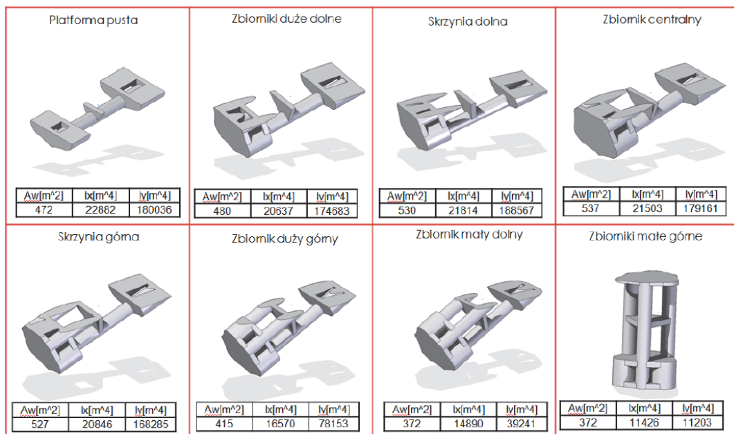
Fig. 6. Changes of platform waterplane during ballasting
