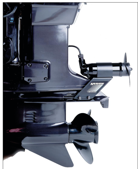
Fig. 2. Electric motor installed on anti-cavitation plate
