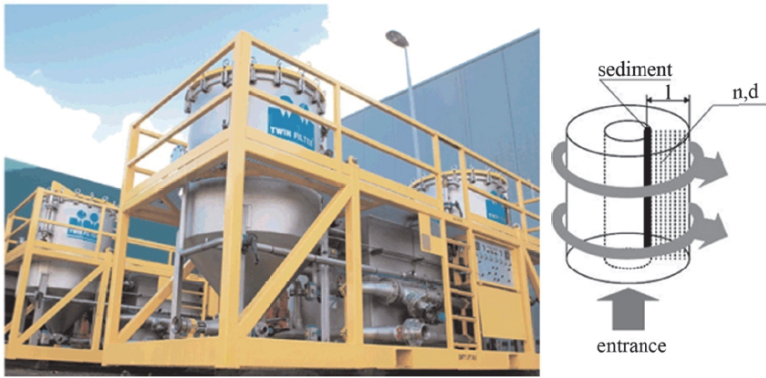
Fig. 7. Scheme and pictures of filter for ballast water treatment [16]
