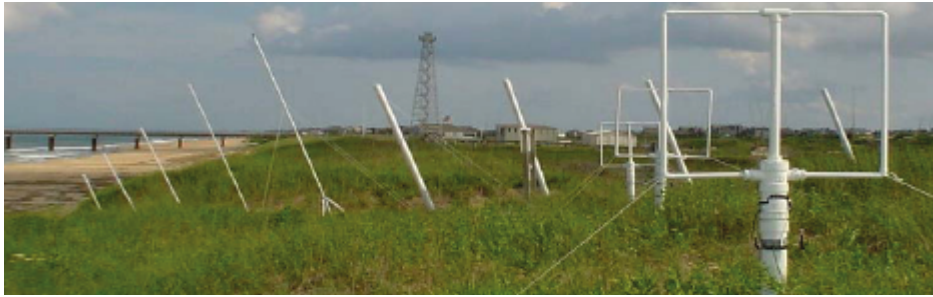
Fig. 2. Multi-Frequency Radar Transmit LPA and Receive LRA – Courtesy of Paper: by Trizna [5]
