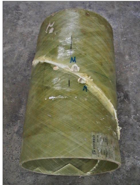
Fig. 9. Destroyed composite coating
