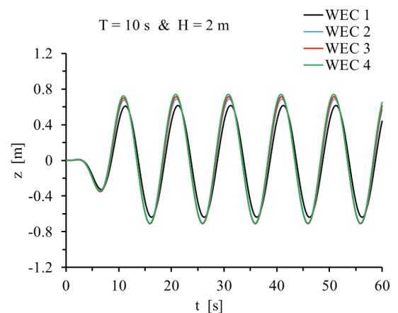
Fig. 16. Comparison of time histories of the WEC heave motion
