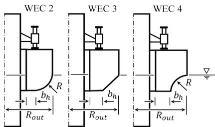
Fig. 4. The sketch of three different types of the WEC system
