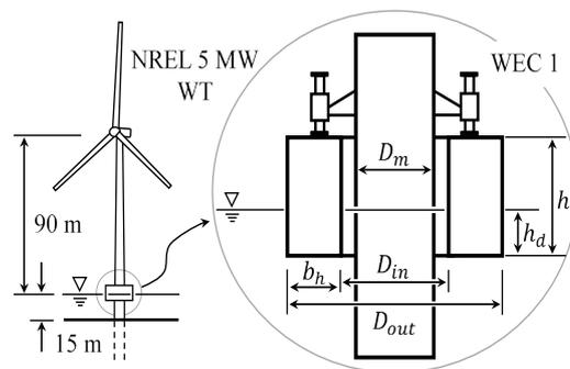
Fig. 2. The overall view of the MWWC system and the sketch of WEC system
