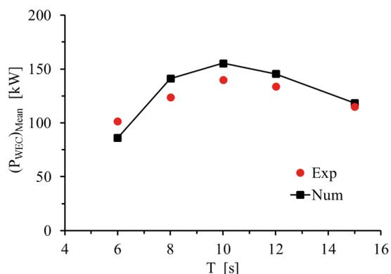
Fig. 10. Comparison of the mean WEC power between experimental data and numerical results for typical regular waves ( $H = 2m$ )
