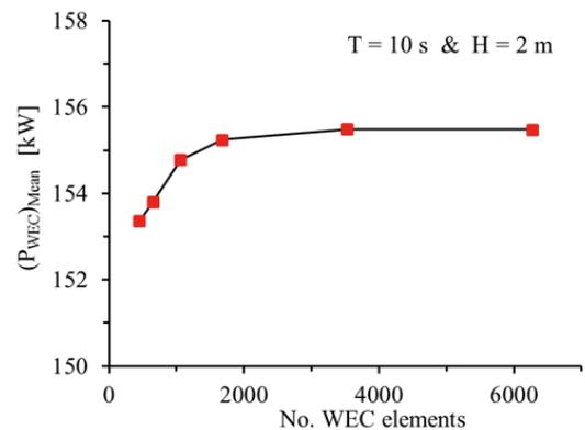
Fig. 7. Mesh study for mean WEC power in typical regular wave case
