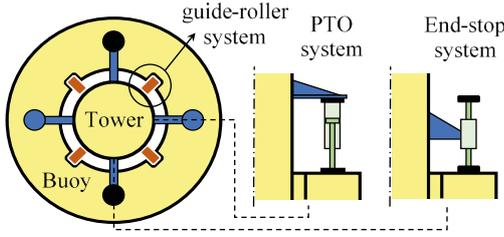
Fig. 3. A sketch of the linear guide-roller system and the end-stop system
