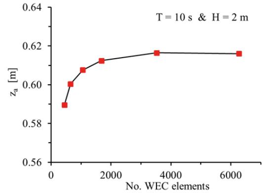
Fig. 6. Mesh study for heave motion of WEC in typical regular wave case
