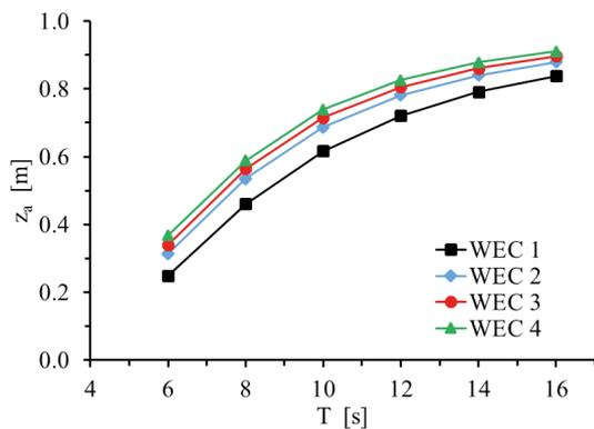
Fig. 13. Comparison of the heave motion for different shapes of WEC ( $H = 2m$ )
