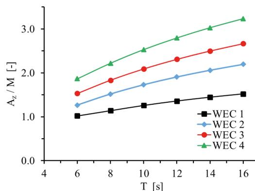
Fig. 11. Comparison of the buoy added mass for different shapes of WEC ( $H = 2m$ )
