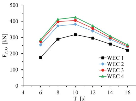
Fig. 14. Comparison of the PTO damping force for different shapes of WEC ( $H = 2m$ )
