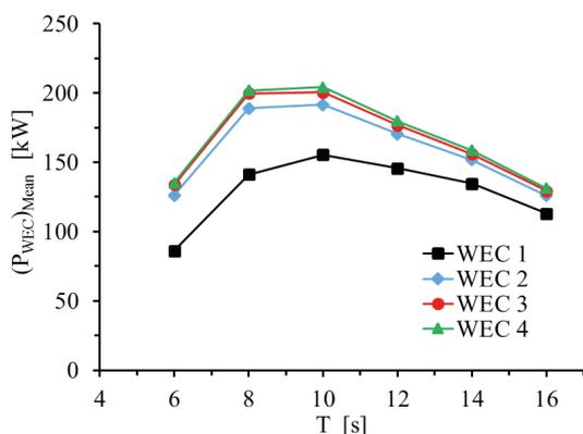
Fig. 15. Comparison of the mean WEC power for different shapes of WEC ( $H = 2m$ )
