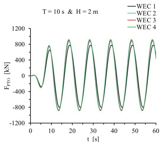
Fig. 17. Comparison of time histories of the PTO damping force
