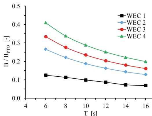
Fig. 12. Comparison of the buoy damping coefficient for different shapes of WEC ( $H = 2m$ )
