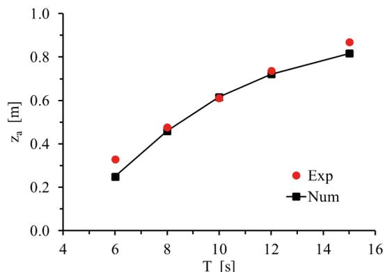
Fig. 8. Comparison of the WEC heave motion between experimental data and numerical results for typical regular waves ( $H = 2m$ )
