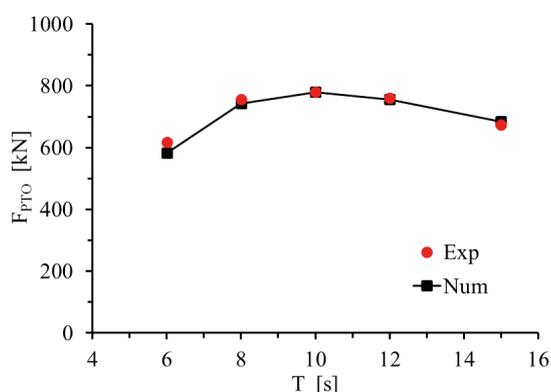
Fig. 9. Comparison of the PTO damping force between experimental data and numerical results for typical regular waves ( $H = 2m$ )
