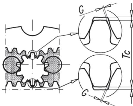
Fig. 7. Tip clearance  $T_c$  and backlash  $G$  [22,27,28]
