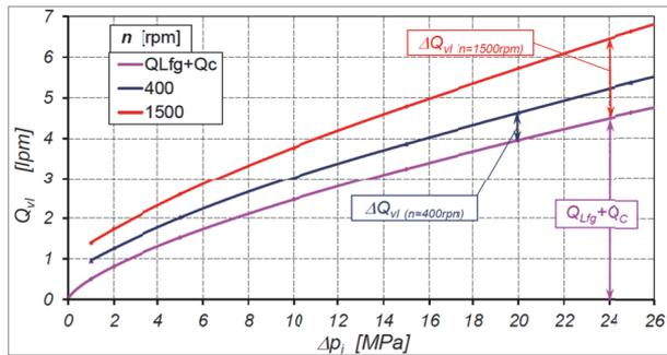
Fig.18. Characteristics of  $Q_{vl}=f(\Delta p_i)$  – result of calculation according to formula (21). Working medium: water
