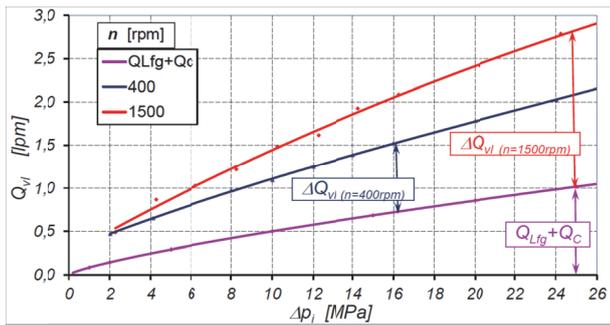
Fig.11. Characteristics of  $Q_{vl}=f(\Delta p_i)$ . Working medium: oil
