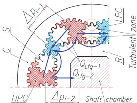
Fig. 6. Flows of liquid in flat clearances [25,26,28]
