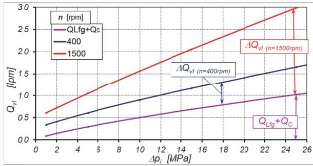
Fig.17. Characteristics of  $Q_{vl}=f(\Delta p_i)$  – the result of calculation according to formula (21). Working medium: oil
