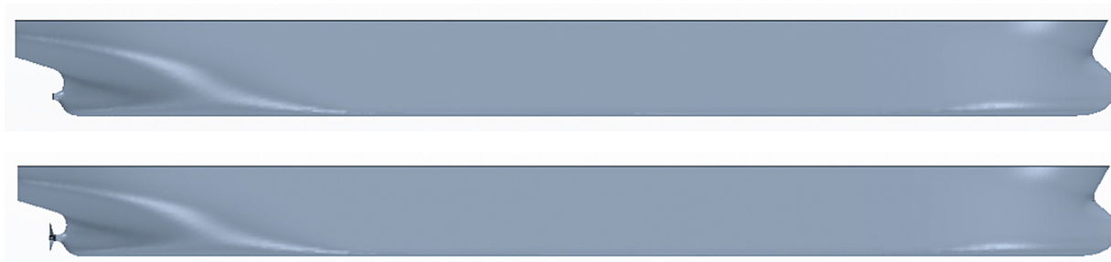
Fig. 1. JBC geometry for simulations of case study “ship resistance” (top) and case study “self-propulsion” in calm water (bottom)
