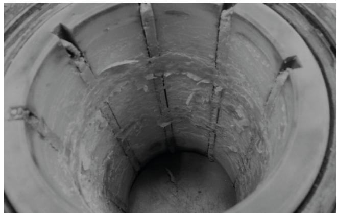
Fig. 7. The bush melt in laboratory conditions, shaft diameter: 100 mm, bush material: elastomer
