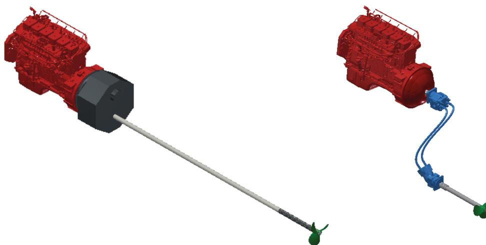
Fig. 1. Visualisation of inland vessel propulsion system (own elaboration)
