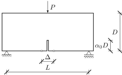
Fig. 3. Boundary conditions and geometry of a beam
