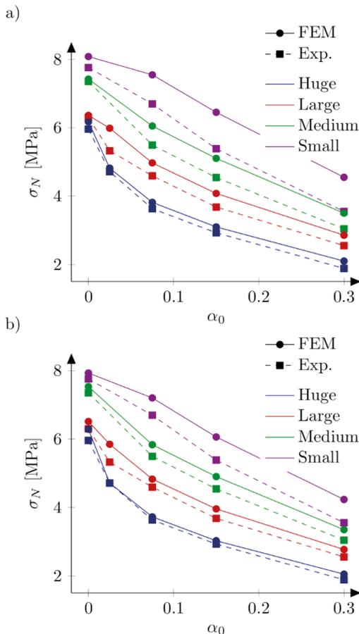
Fig. 8. Nominal (elasto-plasticity calculations) and experimental strengths with the bilinear softening curve,  $f_t=5.0$  MPa,  $G_f=48$  N/m and the characteristic length  $l=5$  mm (a) and  $l=2$  mm (b)
