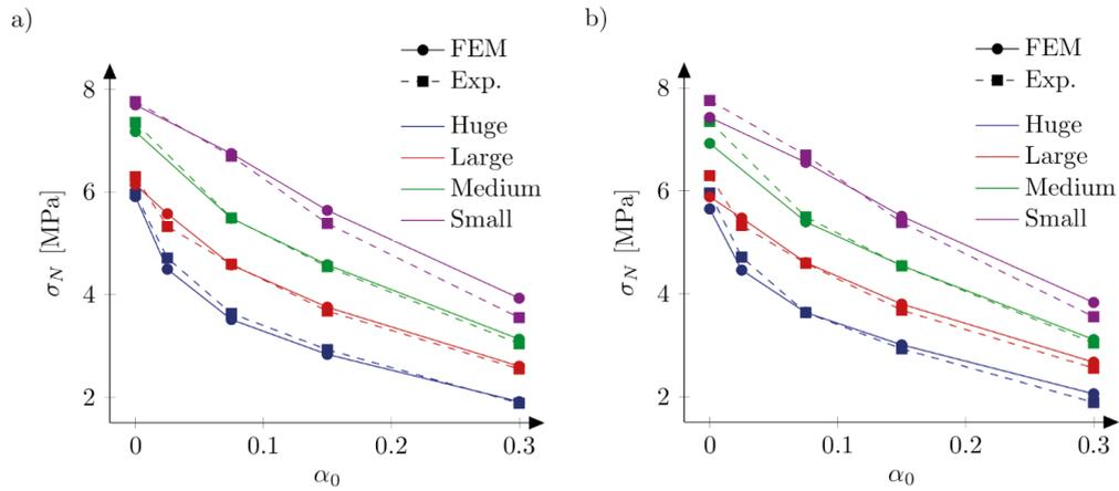
Fig. 6. Nominal (XFEM calculations) and experimental strengths with the bilinear softening curve,  $f_t=5.0$  MPa and  $G_f=48$  N/m (a) and the exponential softening,  $f_t=4.8$  MPa and  $G_f=35$  N/m (b)
