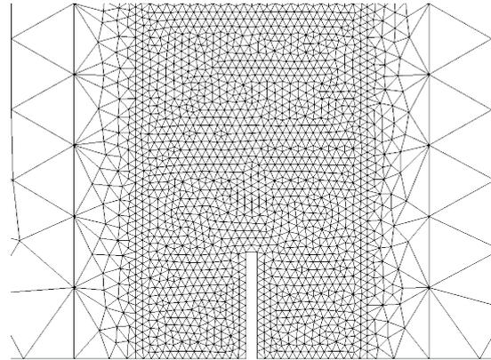
Fig. 4. Exemplary FE mesh around the notch
