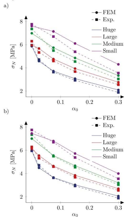
Fig. 9. Nominal (elasto-plasticity calculations) and experimental strengths with the exponential softening curve,  $f_t=4.8$  MPa,  $G_f=35$  N/m and the characteristic length  $l=5$  mm (a) and  $l=2$  mm (b)
