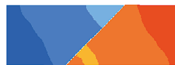
(l) 45° - damage form of pre-crack
