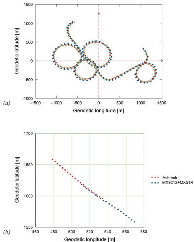
Fig. 5. The trajectories obtained from Ashtech and DGPS receivers in the dynamic trials (a) and indications of the receiver position without taking into consideration the synchronisation of the UTC and GPS times (b) [10]
