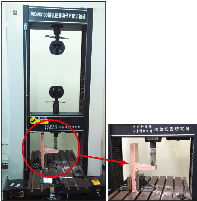
Fig. 6. Mechanical test for the T-type connection specimens
