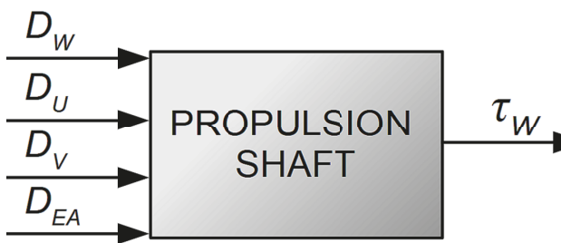
Fig 1. Physical model of propeller shaft fatigue process in a rotating mechanical system developed to determine its durability: D_w – propulsion shaft action associated with mechanical energy conversion in the form of working rotational motion; D_U – propulsion shaft action associated with mechanical energy conversion in the form of heat; D_V – propulsion shaft action associated with mechanical vibration generation; D_{EA} – propulsion shaft action associated with the generation of acoustic emission elastic waves; \tau_w – propeller shaft durability.
