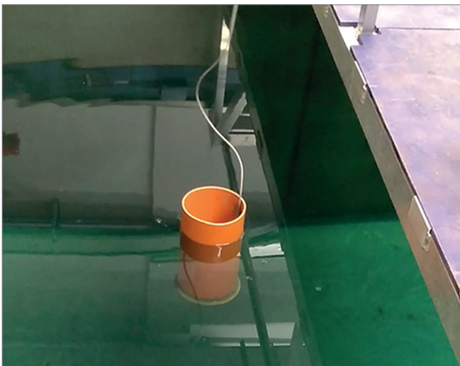
Fig. 6. Model tests of a damping ring cylinder
