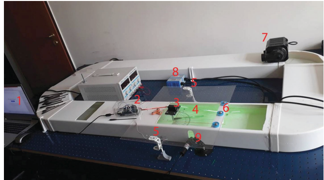
Fig. 5. The laboratory test stand: 1 – PC, 2 – microcontroller unit, 3 – servomotor, 4 – fin, 5 – strain gauges, 6 – ball bearings, 7 – external water pump, 8 – ultrasonic flow meter, 9 – linear laser
