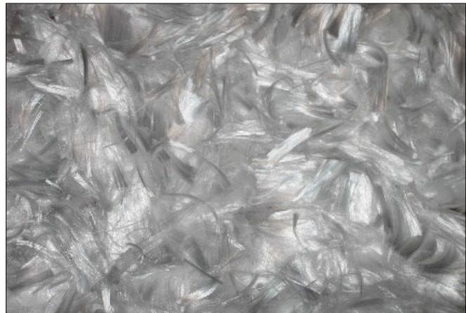
Fig. 3. Polypropylene shrinkage-resistant fibres
