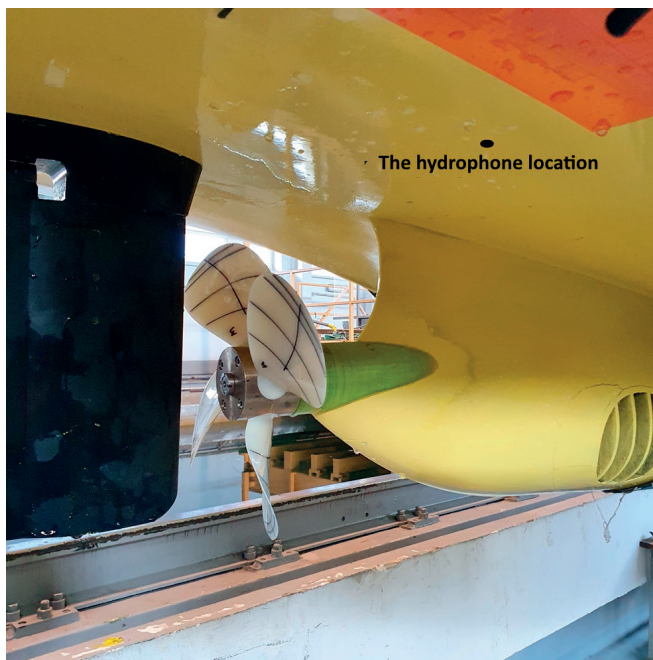
Fig. 6 Attachment of the hydrophone on the underwater part of the hull
